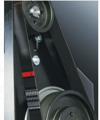
BELT DRIVEN TRANSMISSION The POLY-V belt drive ensures significantly lower power losses and three times the service life compared to standard range "V" type belts fitted to other compressors on the market.
