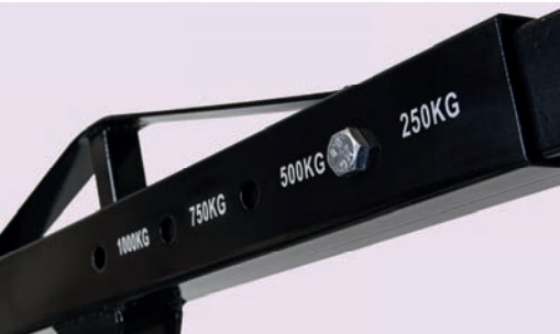
4 hole position boom with indicated weight capacities
