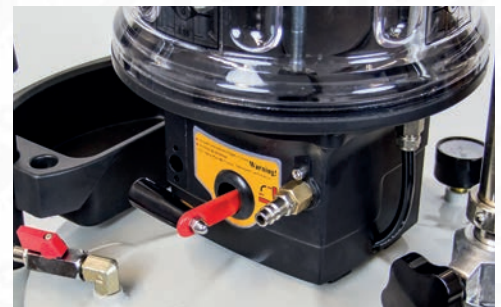
Gravity / Suction switch-over lever
