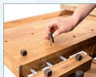
Workpiece holding pegs
