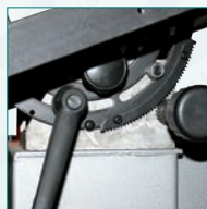
Rack and pinion 45° table tilt
