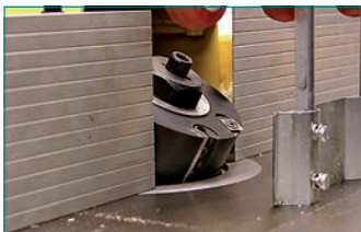
Spindle tilt from -10° to +30°
