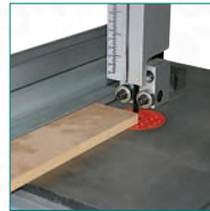
Auxiliary fence for cutting thinner materials
