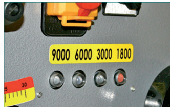
Light display for easy-to-read speed indicator
