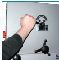
Quick release blade tension
