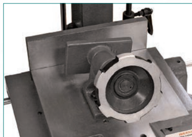
The repositionable cast iron clamp provides a solid hold for a wide range of workpiece sizes
