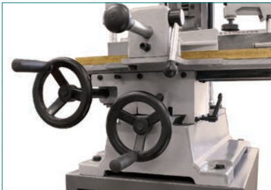
Multi-height, depth table adjustment
